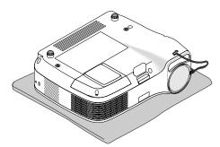
2. Loosen the lamp cover screw until the screwdriver goes into a freewheeling condition and remove the lamp cover.
